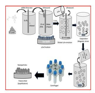
$\begin{tabular}{ll} \textbf{Figure 1.} & \textbf{Nanoparticles preparation procedure with Eudragit RL 100} \\ \textbf{polymer} \\ \end{tabular}$
