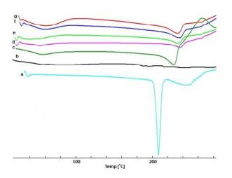
**Figure 4.** DSC thermogram of Ketotifen fumarate (a); Eudragit RL 100 (b); PVA (c); blank NPs of  $F_2$  (d);  $F_1$  (KF:EU) 1:7.5 ratio (e);  $F_2$  (KF:EU) 1:10 ratio (f);  $F_3$  (KF:EU) 1:10 ratio (g), respectively
