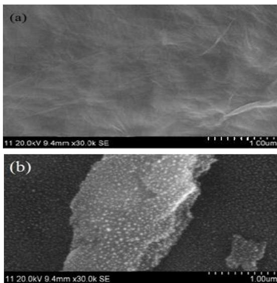
Fig. 1. SEM images of (a) GO and (b) GO/TiO<sub>2</sub>
