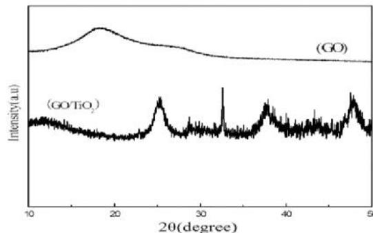
Fig. 3. X-ray diffraction patterns of GO and GO/TiO<sub>2</sub>
