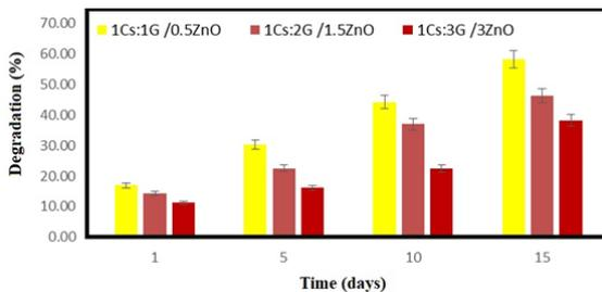
Fig. 5. Biodegradation process of coated three-dimensional scaffolds
