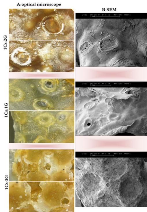
Fig. 2. Examination of morphology using 80x optical microscope and SEM for 3D scaffolds
