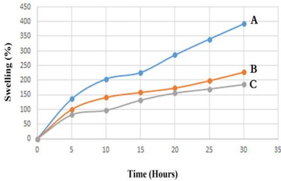
Fig. 4. Swelling percentage diagram of 3D scaffolds without coating, A) 1Cs:3G, B) 1Cs:2G, C) 1Cs:1G
