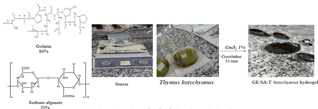
Fig.1. Schematic synthesis of GE/SA / *T. kotschyanus* hydrogel
