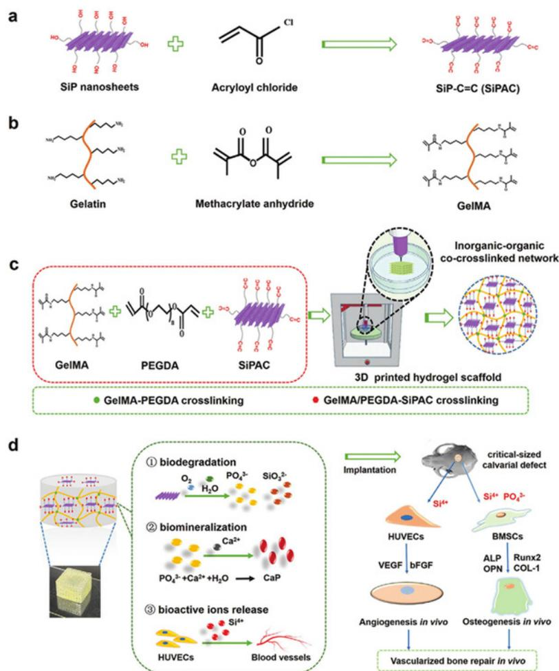
Fig. 3. Schematic representation of the creation of 3D printable hydrogel scaffolds using SiP nanosheets and their use in the regeneration of vascularized bone (63) with permission from Wiley (License Number: 5593590649991), 2023
