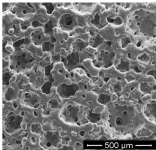
Fig. 2. This scaffold was obtained by gel-cast foaming, freeze-drying, and sintering [51].
