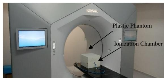
Figure 2. Ionization Chamber placed inside the Plastic Phantom
