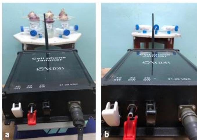
Figure 1. The mobile phone jammer and the circular plastic tray show the experimental setup and the principle of exposure to mobile phone electromagnetic radiofrequency field at 1800 MHz, and a SAR value of 0.27 W/ kg. a. Each onion bulb is placed in the mouth of a 50 ml glass baker. b. Each mouse was placed inside a separate perforated 50 ml polypropylene tube with the head oriented towards the center
