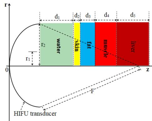
Figure 1. Simulation model of multi-layer biological tissue irradiated by HIFU
