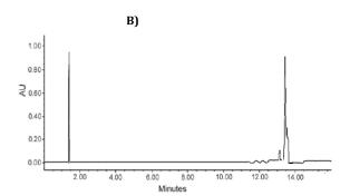
Figure 1. HPLC analysis of fraction 10 (A) and standard luteolin (B). Chromatographic conditions: RPC18 column, mobile phase: methanol/acetone/water = 70/20/10 (v/v/v) at 1.5 mL min<sup>-1</sup>
