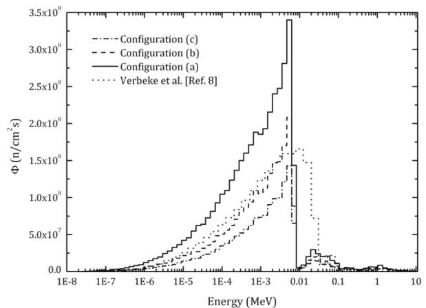
Figure 2. Neutron spectrum calculated at the beam port of three designed BSAs and the proposed configuration of Ref. [8].
