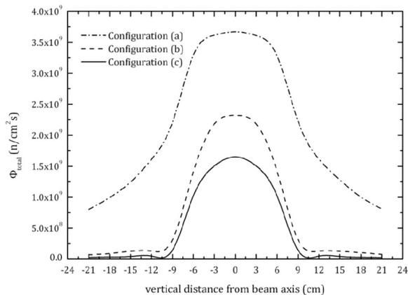
Figure 3. Total neutron flux calculated at 1 cm from beam port of configurations (a), (b), and (c) versus different vertical distances.
