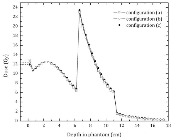
Figure 5. Total delivered dose to different depths in the simulated head phantom due to the designed beams related to three proposed configurations.
