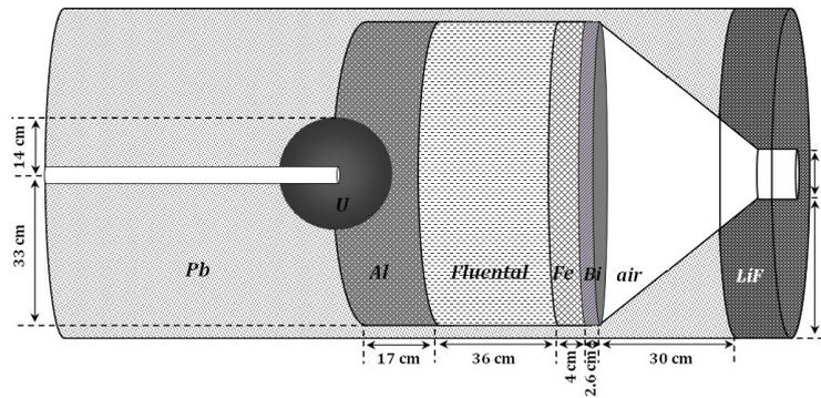
Figure 1. Designed BSA: Natural uranium as neutron multiplier, Al and Fluental as moderators, Fe as fast neutron filter, Bi as gamma filter, and Pb as reflector and collimator. LiF thickness in configurations (a), (b), and (c) are 0, 4, and 7 cm, respectively.
