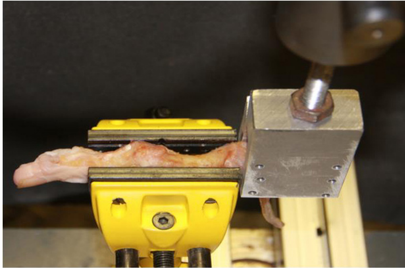
Figure 4. Each thumb was clamped tightly and subjected to mechanical testing. The clamp on the right (grey) applied deflection to the trapezium to recreate physiological movements. In this example, dorsal subluxation (extension) is tested.
